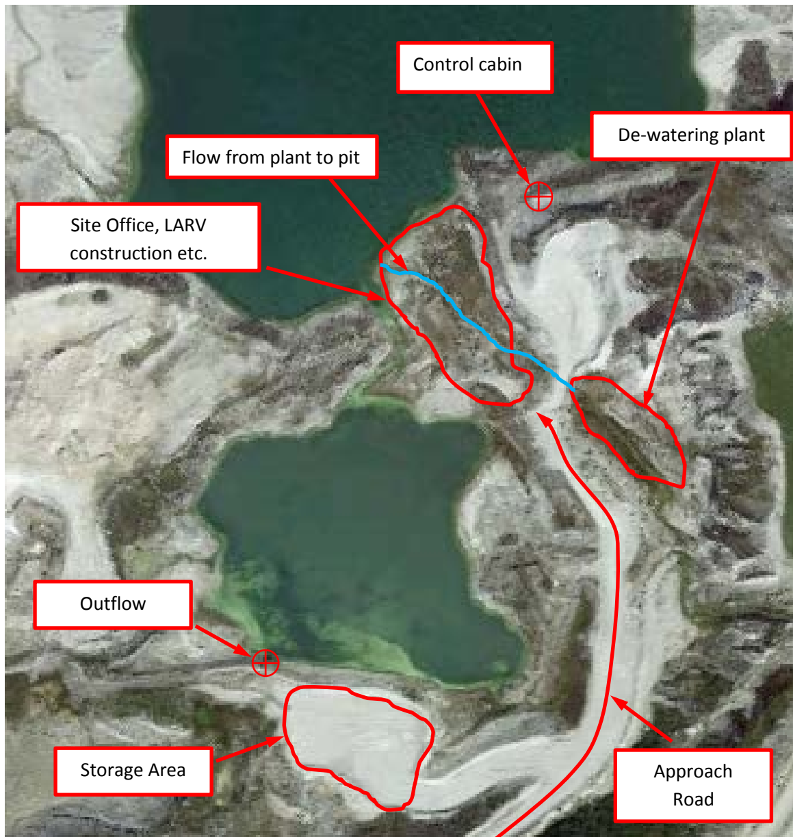
Figure 8 – Whitehill Yeo Pit – Equipment Location
